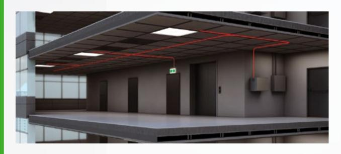
LED technology in emergency lighting systems has increased efficacy and decreased energy requirements so that an entire floor or large area can be powered by a Mini Inverter. Today's highly efficient Mini Inverter-powered emergency lighting systems consume less energy and require fewer units for maximum economy and reliability.
