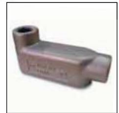
The BlueKote® conduit body still has a glossy sheen and no evidence of salt adhesion or penetration after the same salt fog test.
