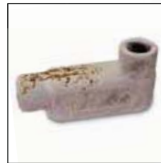
After a 500-hour 5% salt fog test, the standard galvanized iron conduit body has severe salt adhesion and significant rusting.
