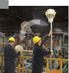
The quick pole assembly blocks at a 90° angle.
