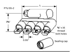
Note: All transformer connectors include a jam nut and EPDM rubbing bushing stud cover. All outlets except one are factory-sealed with removable sealing caps. For complete assembly with CS 2011 insulating rockets, add "-AWR" suffix to the catalog number. For other accessories, see pages C44–C45.
